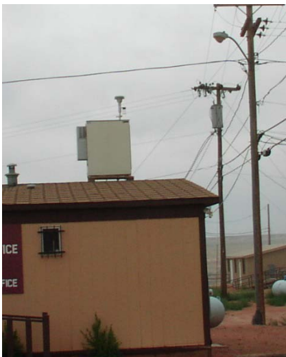
This photo is the TEOM setup, collecting PM 10 collecting data at Tuba City, Arizona.
