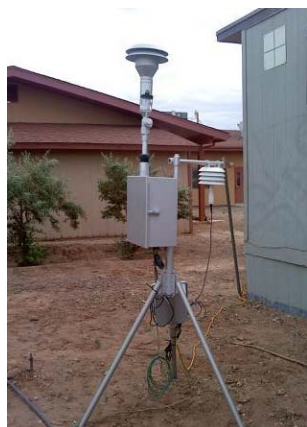
This picture is the E-BAM setup, collecting PM 2.5 data at Leupp, Arizona.
